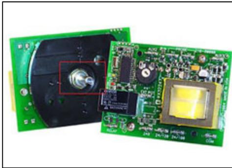
**Overview:** ISL was asked, by a world-leading fast food chain, to take an existing potentiometer that the customer was having failures with, and develop a replacement that would withstand the harsh environment of a commercial kitchen.
